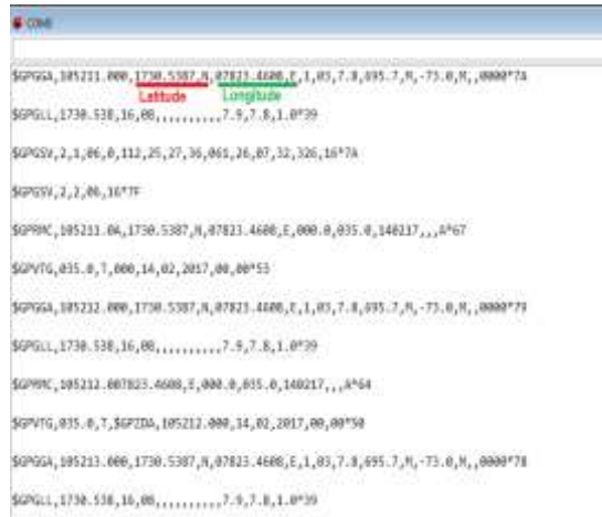
Fig. 11 Data received by the GPS Receiver
